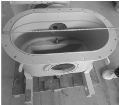
图 14 防爆型互感器的油箱设计 Fig. 14 Oil tank design of explosion-proof instrument transformer
